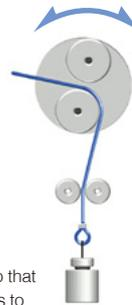
As shown above, fix the core wire so that it does not move, bend it 90 degrees to the left or right, and confirm that no wire breakage occurs.
