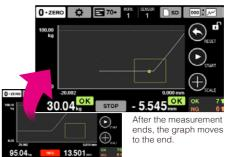
During measurement (graph drawing from the left end)
