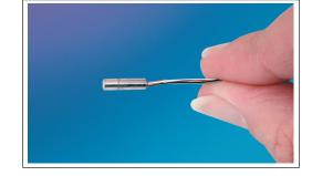
The XCL-072 design features Kulite's patented leadless technology. This allows for a very rugged package suited for probes, pressure rakes and other similar test set ups. This transducer is well suited for both dynamic and static pressure measurements in benign or harsh environments.
