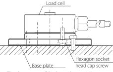
The dimensions of the base plate and the screws are shown in the table below.
